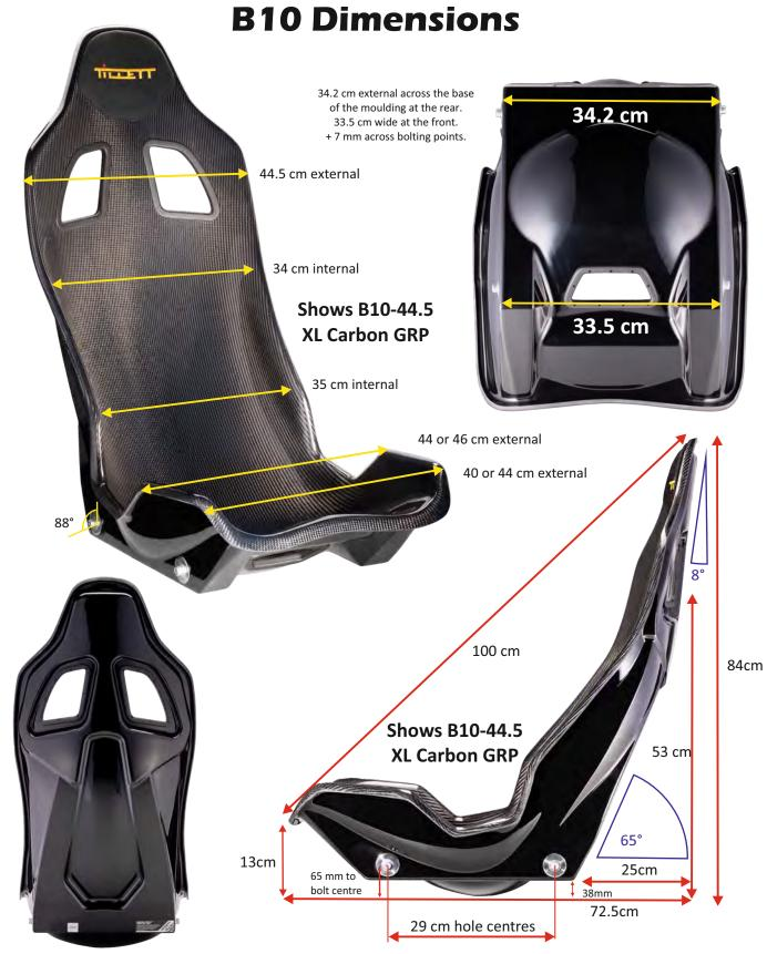
Tillett Racing Seats Styles Close, Sittingbourne, Kent, ME10 3BF, England Tel : 01795 420 312 customerservice@tillett.co.uk www.tillett.co.uk The B10 seat can use the bracket sets STBi, STBO, TBFIA, VTBi, VTBO, and Elise brackets EBR, EBR 17+, EBS, EBP. These brackets have a 2° from vertical angle, which matches the side of the seat. Brackets which do not match this angle will unduly stress the composite.
